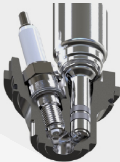
>> Injector & spark plug configuration in active system
